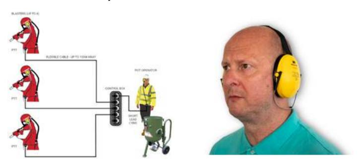
The Wired Communication System is a reliable and economical way to ensure vital communication between a blast pot operator and up to four blasters. The wired system includes communication headsets, a control box and high-quality noiseless instrument cable.
